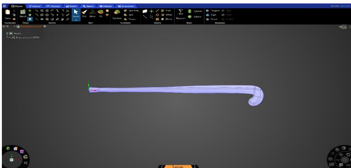
Figure 22: CAD geometry of the hockey stick displaced to the origin and rotated to align with the y-plane.
