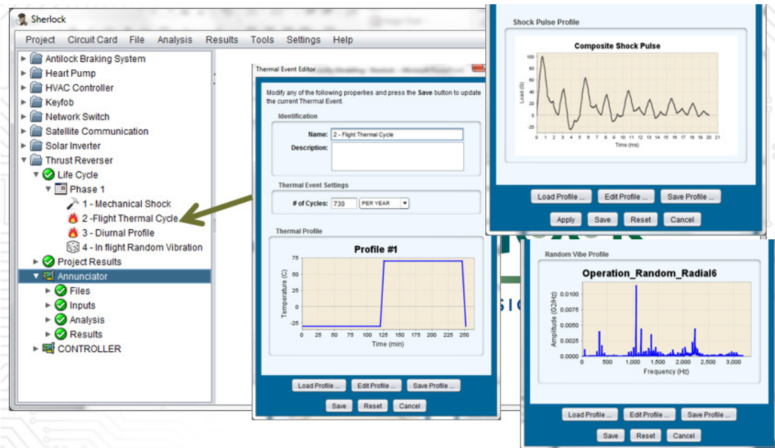
Figure 3. Thermal shock, mechanical shock and random vibration stresses in Sherlock
