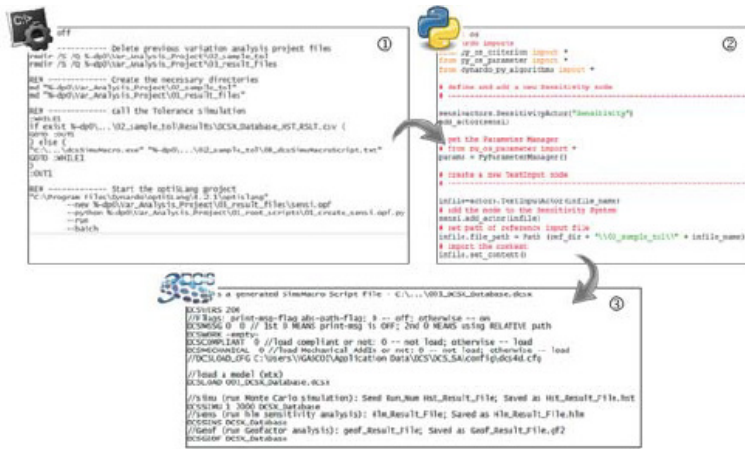
Figure 7 *.cmd call, the Python script creates optiSLang project, the tolerance simulation in batch call.
