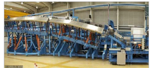
Figure 2. Test rig of the A380. In the front, drive systems and load cylinders to simulate the air load.
