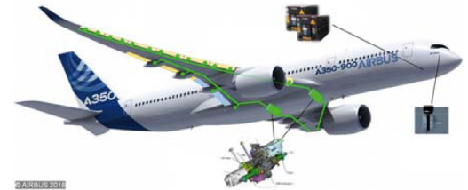
Figure 1. Principle structure of the High-Lift System (HLS).
