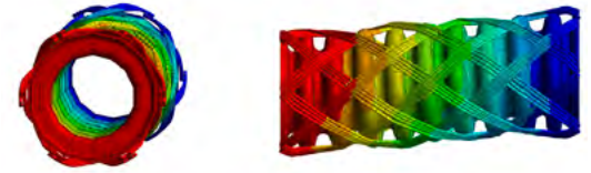
Figure 34. Tri-axial deflection - single braid layer - front and side views.
