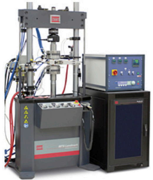
MTS Landmark® test system configured for thermomechanical fatigue (TMF) testing.
