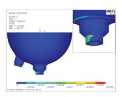
Creep damage contour plot after implementing the Ansys subroutine.
