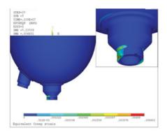
Creep strain contour plot after implementing the Ansys subroutine.
