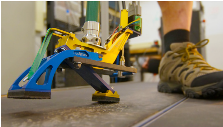
HuMoTech's prosthetic foot worn by a user with unilateral transtibial amputation.
