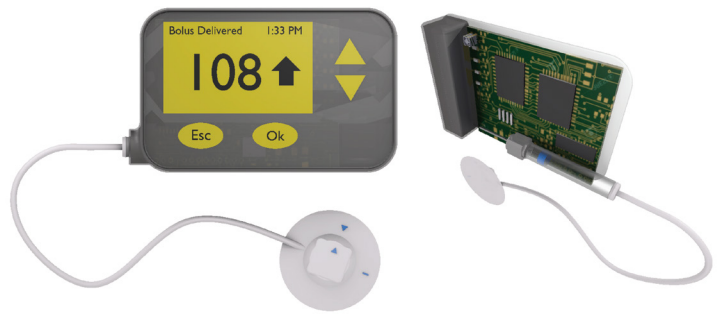
Figure 3. External view (left) and internal view (right) of an insulin pump digitally simulated on the Ansys platform.
