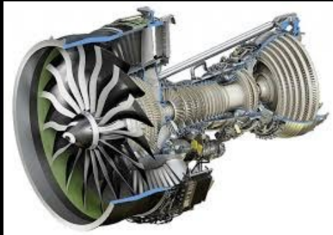
GE Aviation – LEAP engine FADEC for Airbus A320 Neo, Boeing 737 Max, COMAC C919 (1 st flight 2016)
