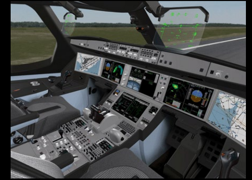
Thales Aerospace – Airbus A350 Cockpit Display System (1 st flight 2013)
