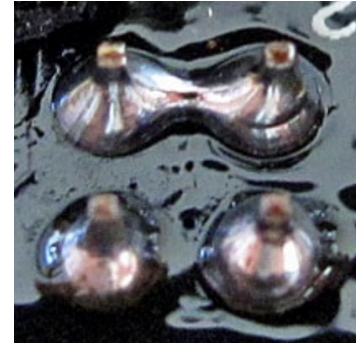
Bridging of two solder balls Surfacemountprocess.com
