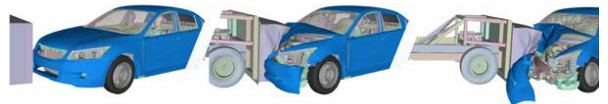
A frontal offset crashworthiness evaluation is a common use of Ansys LS-DYNA nonlinear dynamics structural simulation software.
