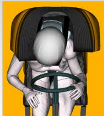
Helmet foam simulation, right-side impact, THUMS 50th percentile male
