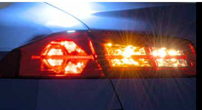
Figure 3. Tail lamp simulation results from Ansys Speos software.
