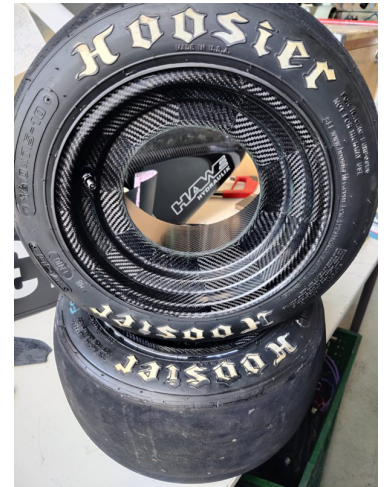
Inflated tires on optimized CFRP rim
