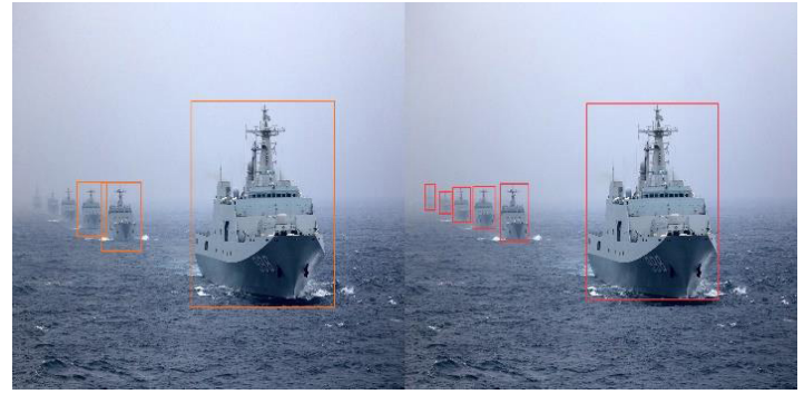
Detection results with the models trained on synthetic AVxcelerate Sensors images (left) and on the hybrid dataset (synthetic and real images, right)
