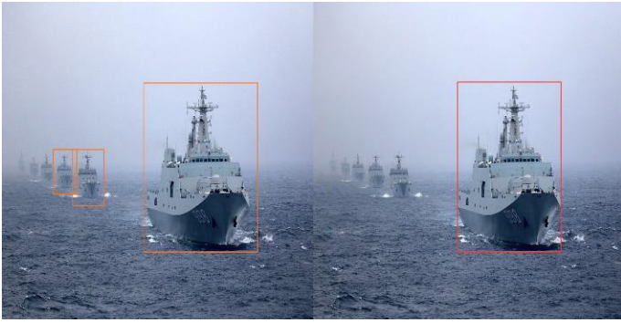
Detection results with the models trained on synthetic AVxcelerate Sensors images (left) and real images (right)
