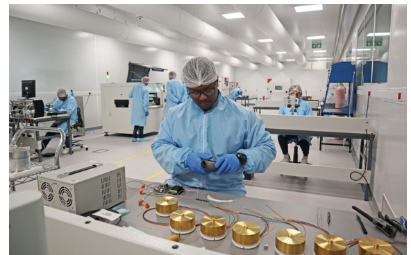
Figure 2. Reaction wheel production in cleanroom
