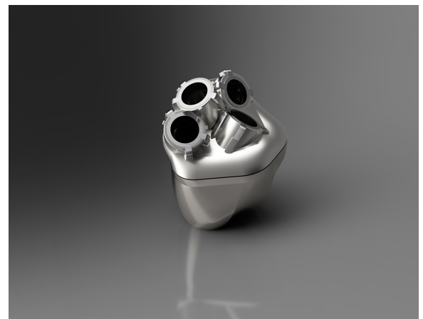
Rendering of the 2024 TAH casing in Autodesk Inventor
