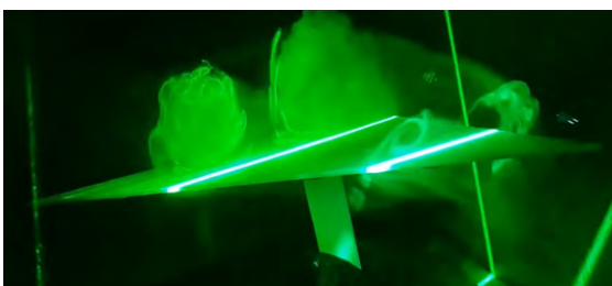
Flow visualization around a delta wing
