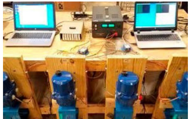
Figure 2: Mechanical ALT of flow control valves.
