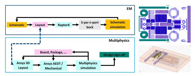
In Ampleon's electromagnetic and multiphysics design flow, a first-order simulation is performed at the schematic level, then the generated layout is simulated in Ansys RaptorX $^{\text{\tiny{M}}}$  to create an S-parameter block for a new schematic simulation. The layout is imported into Ansys Electronics Desktop $^{\text{\tiny{M}}}$  for Ansys Mechanical $^{\text{\tiny{M}}}$  system-level multiphysics simulations.
