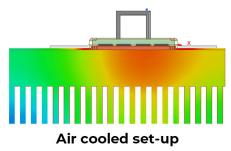
Ansys multiphysics simulations help Ampleon engineers visualize temperature distributions at the system level and ensure that values remain within the safe limits.
