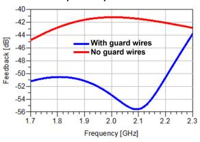
Electromagnetic simulations with Ansys Electronics Desktop™ help Ampleon identify measures to reduce the input-to-output coupling in packaged devices. This coupling is often due to the magnetic field generated by the wires at the output which flow through the wires at the input. A possible solution is to add "guard" wires at the side of the transistor to reduce the outflowing field. This patented solution significantly reduces coupling.
