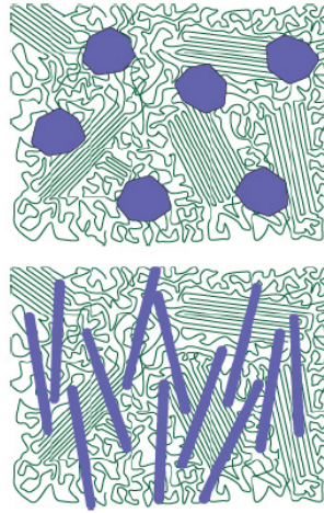
Figure 9. A polymer with particulate and fiber fillers
