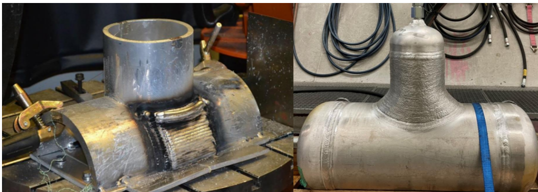
Figure 2. Linde applied Ansys optiSLang to conduct a thorough economic analysis of an additive arc manufacturing process for aluminum components in plant and pressure vessel construction.
