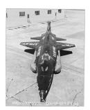
later modified, the basic X-15 outer skin consisted of a nickel-chrome alloy called Inconel X, employed in a heat sink structure to withstand the results of aerodynamic heating when the aircraft was flying within the atmosphere. The cabin was made of aluminum and was isolated from the outer structure to keep it cool.
