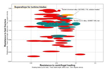
Focusing on the material classes that perform best in resistance to fast fracture and to centrifugal loading, a custom subset of cobalt-base as well as nickel-chromium and nickel-cobalt, we can quickly make an overview plot and identify the main candidates. As expected, the Nickel-Chromium superalloy, Inconel 718 is one of the best materials in both these objectives. That holds true also for cost performance, as seen below. A comparison table shows how several key properties are compared.
