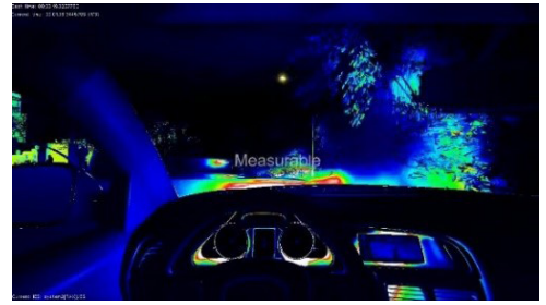
Illumination maps in false colors demonstrate the performance measurement of any illumination system.
