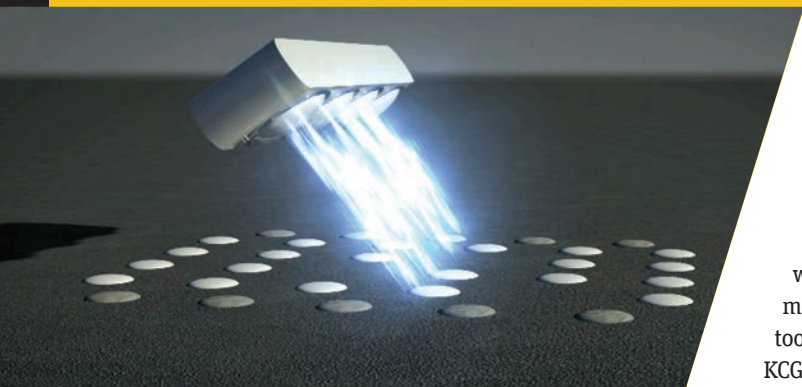
Four-radar RPS reading paint dot bit pattern on road
