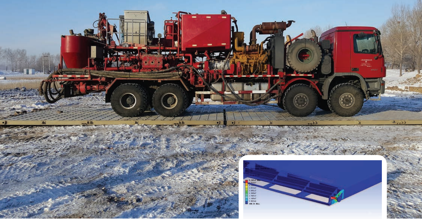
Four base boxes under a piece of machinery
