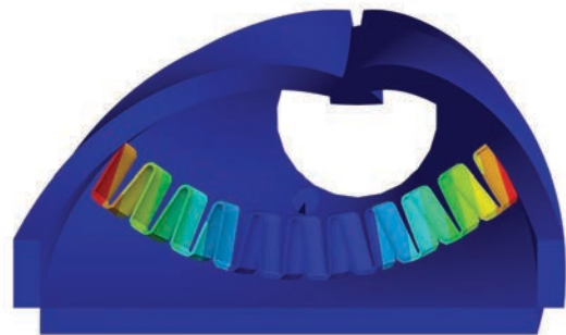
Second-generation rolling die correctly seals tubes.
