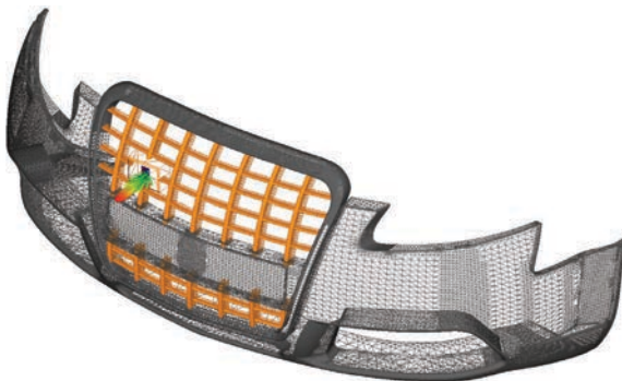
A radar sensor array model is installed in a proposed automobile fascia (left), and the ANSYS HFSS SBR+ shooting and bouncing rays EM field solver is applied to model the installation interactions. The HFSS finite-element simulation for the radar sensor antenna system is shown in the proper installation location, and a subset of rays employed by the HFSS SBR+ simulation is shown at an exit angle of 80 degrees.
