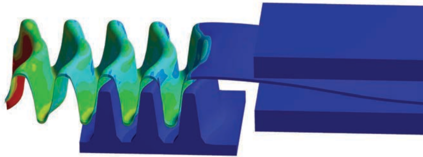
Simulation guided engineers in developing a new progressive die that produces good fins.
