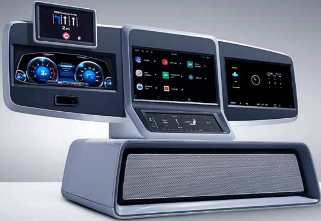
State-of-the-art digital cockpit domain controller containing one system on a chip (SoC) driving five displays
