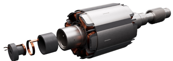
ZF's electric motor is uniquely compact due to its innovative rotor design: the energy for the magnetic field in the rotor is generated by coils whose current is transmitted via an inductive exciter inside the rotor shaft.
