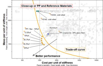
When investigating this synthesized hybrid material, the so-called **Part Cost Estimator** quickly estimates the cost to manufacture a component and compare different classes of materials and processing routes. Thus, not only the cost of the materials is considered but the combination of materials and manufacturing.
